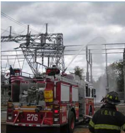
This incident led Con Edison to evaluate various firefighting agents for transformer fires. Only one agent was capable of being applied to 345 kV with imperceptible electrical feedback to the nozzle, F-500 Encapsulator Agent. Today, Con Edison recommends F-500 Encapsulator for transformer fires. After the power is removed, F-500 EA can be safely applied without fear of electrical feedback to the nozzle if the stream comes into contact with nearby energized peripheral equipment.
