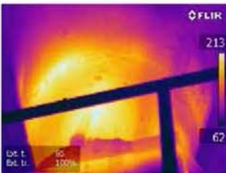
Steel silo fire, internal temperature 100°F readings on camera.
