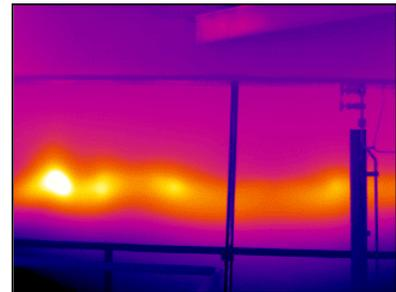
C. Map coal bunker, hopper, or silo fire area and plot temperatures to determine location and intensity of fire. Some high-end thermal cameras are equipped with software that will produce thermographic images with temperatures correctly plotted on the image.
