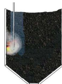
The piercing rod injects F-500 EA. The thermal imaging camera will confirm the fire is out.
