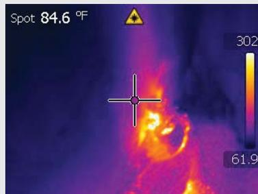
A thermal imaging camera is the key to locating hot spots and is included with each Piercing Rod System. The picture shows an actual hot spot image. Knowing the location of the hot spot will guide the piercing rod team as they insert the piercing rod.
