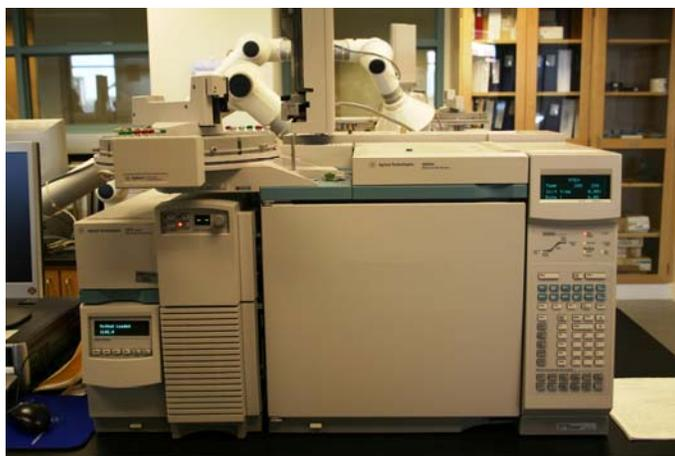
*The Agilent Technologies 6890N Network GC System is use by lab technicians to test samples from the study and provide the supporting data for this report.*
