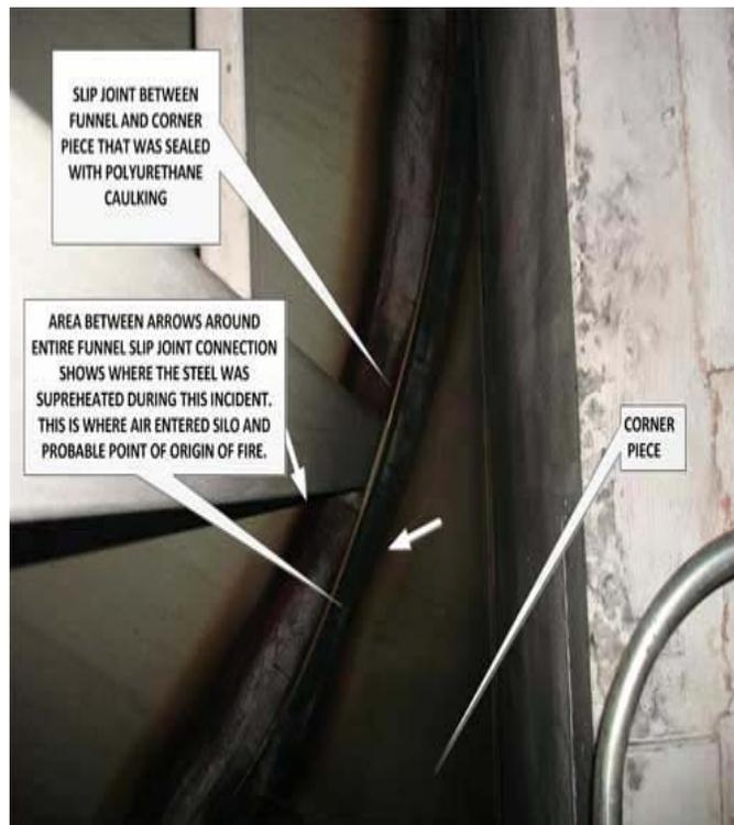
**Photo 3. Shows lines of demarcation where fire was burning inside silo around the slip joint between the funnel and the corner pieces.
