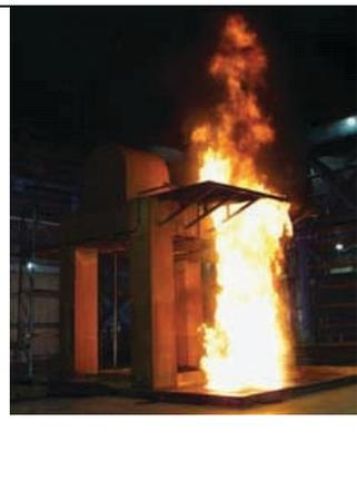
FM Global's generator mock-up, simulates oil spray, pool, and pressurized 3-dimensional fires – typical components of a turbine lube oil fire scenario. In a recent study, over a 15-year period, FM Global found that fire protection deficiencies for lube-oil systems were a major factor in 17 large turbine building fires.
